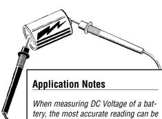
When measuring DC Voltage of a battery, the most accurate reading can be attained by testing the battery under load. To accomplish this, follow steps 1 through 4 shown on page 15 and the following (with the battery in holder and device turned on):
